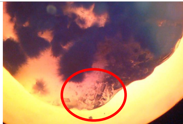
FIGURE 2. Lysozyme crystals and NaCl crystals in 3.0 M NaCl and 4.8 pH solution with Izit dye.
